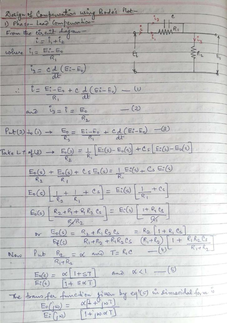
The steady state performance of the T.F. is governed by low freq. characteristics and formient performance is governed by high freq. Characteristics, for simultaneous satisfaction of tooms cut & steady state performance, the Bode Plot must be rechaped so that the high freq. portion of the first satisfies the phase margin requirement and low forg. postion satisfies the Kr requirement. [ E. (w)/E Pole zero and Rode Plotmagnitude
