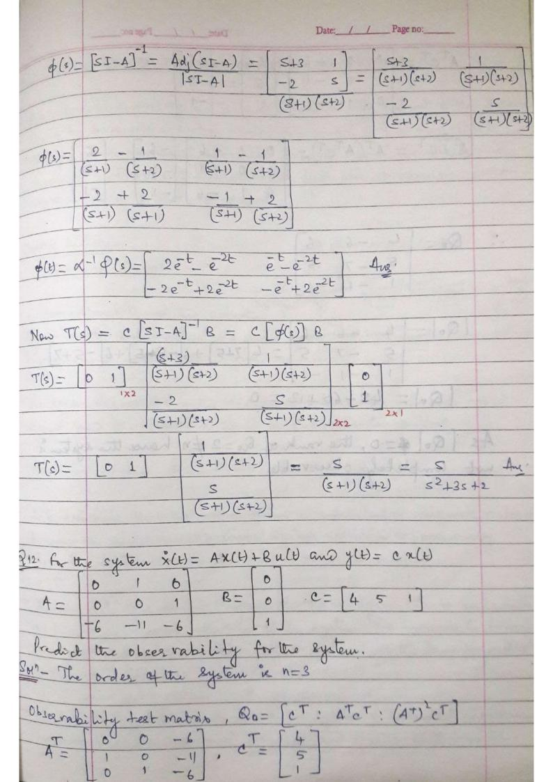
$$(A^{T})^{2}c^{T} = A^{T}(A^{T}c^{T}) = \begin{bmatrix} 0 & 0 & -6 \\ 1 & 0 & -11 \\ 0 & 1 & -6 \end{bmatrix} \begin{bmatrix} -6 \\ -1 \end{bmatrix} = \begin{bmatrix} 6 \\ 5 \\ -1 \end{bmatrix}$$
